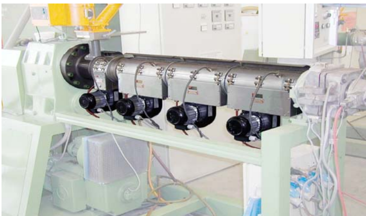
Fig. 5: Plasticising unit for extruder retrofit
