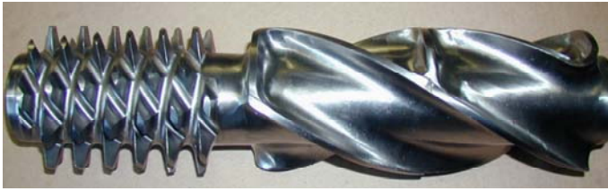
Fig. 1: Homogenizing section of a barrier-mixing screw
